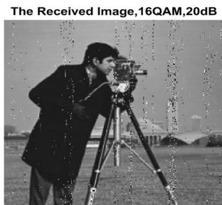
(c) The Rx. Image with 16QAM, and SNR = 20dB
