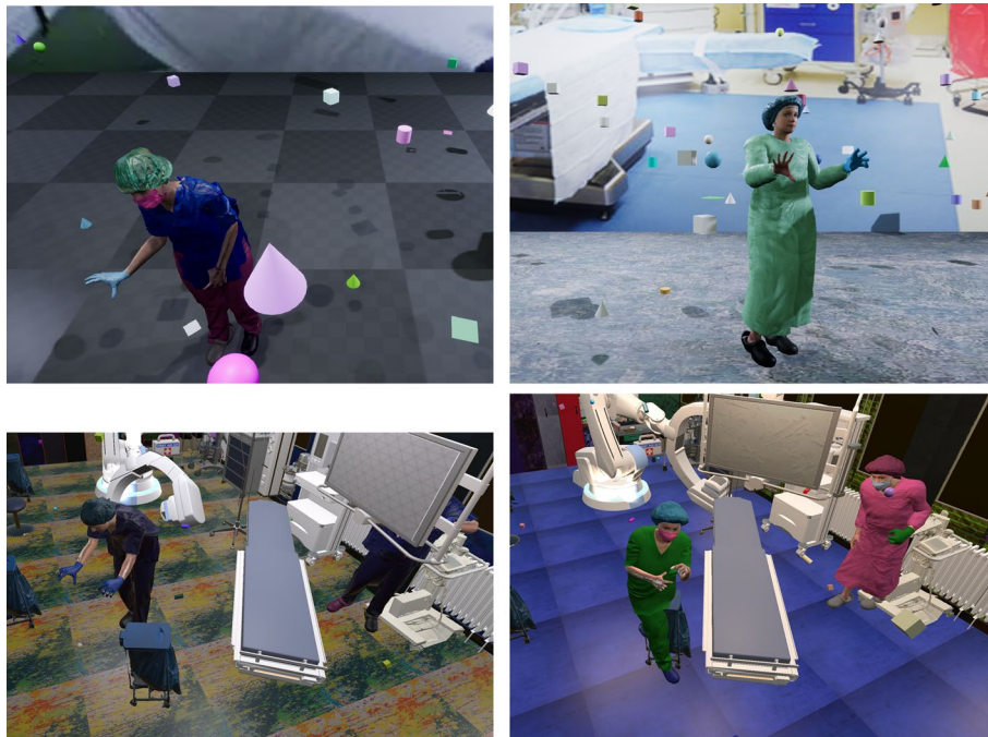
Fig. 4 Examples of synthetic RGB image data from Domain Randomization (DR) and Structured Domain Randomization (SDR) datasets (top: DR, bottom: SDR, left: SCANS, right: CAD)
