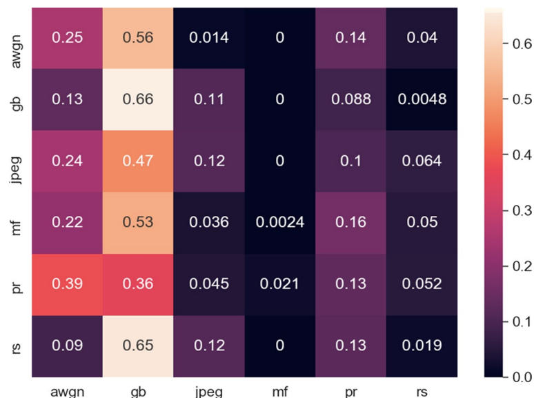
Fig. 4 Confusion matrix for Bayar2016 trained on original IFSTC, evaluated on Xerox1 (see Table 2, Xerox1). We note that despite the high reported validation accuracy on the original data set, the model struggles to distinguish between the classes after printing and scanning
